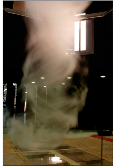
Figure 3.5. A laboratory simulation of a tornado.
