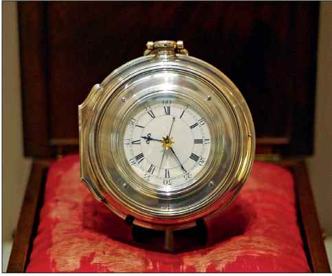
Figure 2.4. One of Harrison's marine chronometers. The invention of accurate clocks in the 1700s enabled navigators to make accurate plots of their positions at sea for the first time.
