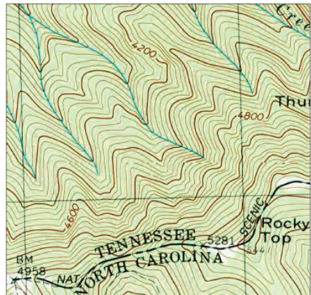
Figure 2.34. Principle 3—Contour lines make a V where they cross streams, with the V pointing upstream.
