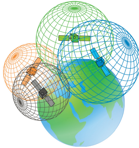
Figure 2.9. The spheres represent different distances from GPS satellites. The point where the surfaces of all four spheres intersect is the location of the receiver.
