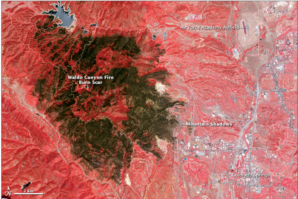
Figure 2.24. Satellite imagery is used to analyze damage to forests due to wildfires. In this image, red is healthy vegetation, gray is bare ground or man-made features, and dark brown is the burn scar from a wildfire.
