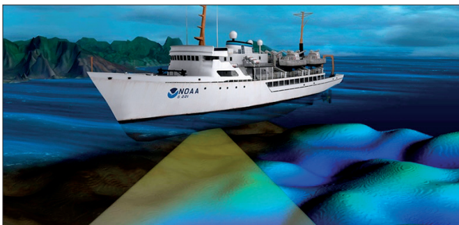
Figure 2.26. Echo sounding uses sound waves transmitted through water to determine water depth.
