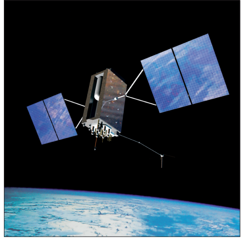
Figure 2.6. A Global Positioning System (GPS) satellite, with solar panels to supply it with electricity.
